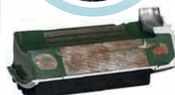
Insulated motor winding cross section
